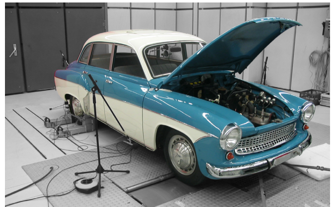
Figure 1: Measured Wartburg 311 on a vehicle dynamometer.
